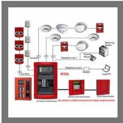
Fire alarm Systems Service
