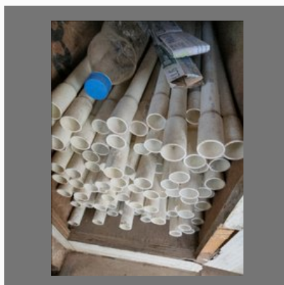
Electrical PVC Pipes
