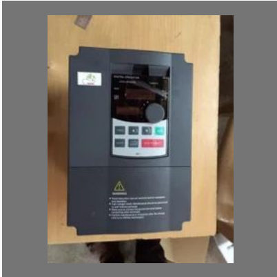
Solar Motor Controller
