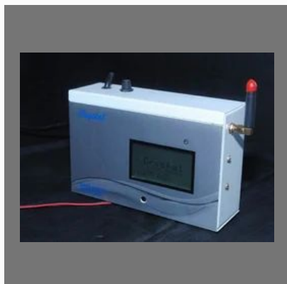
Prepaid Energy Meter
