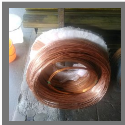
Bare Copper Wire
