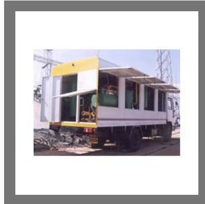
Transformer Oil Conditioning Plant
