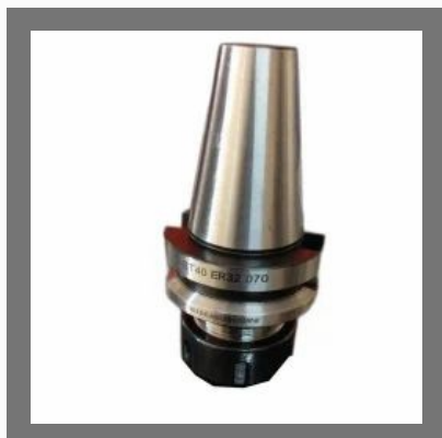
BT40 ER32 070 Adapter G6.3 RPM 15000
