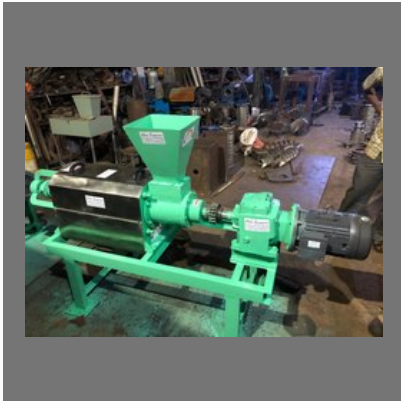
Cow Dung Dewatering System
