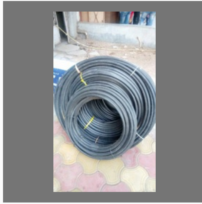
Electrical PVC Pipe
