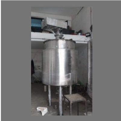
Paint Manufacturing Vessel
