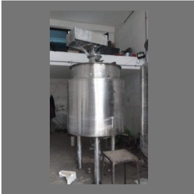
Liquid Mixing Tank
