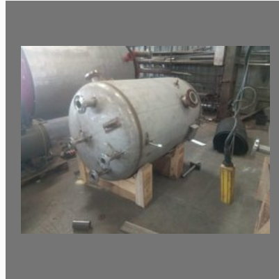
Above Ground Diesel Storage Tank
