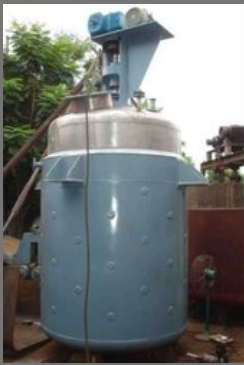
OUTSIDE HEATING COIL PRESSURE VESSEL
