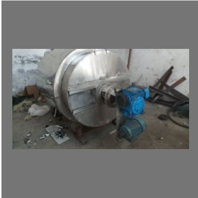
SS Chemical Mixing Tank
