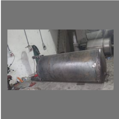
Chemical Receiver Tank
