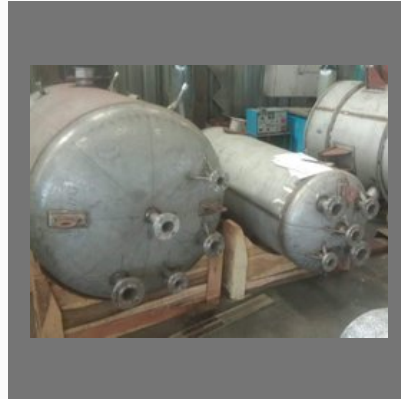
STAINLESS STEEL STORAGE TANK
