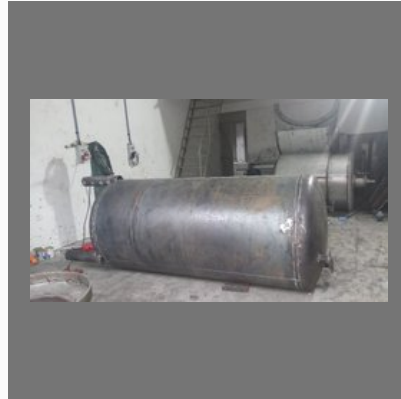
FO STORAGE TANK
