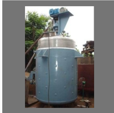
OUTSIDE HEATING COIL PRESSURE VESSEL
