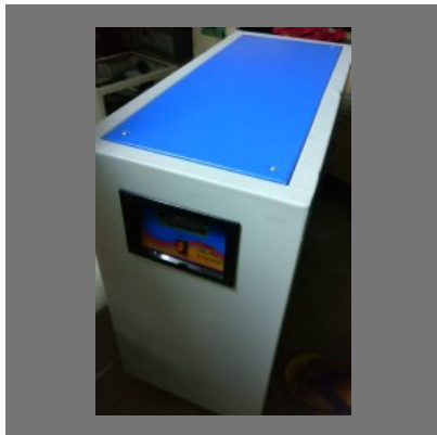
DSP Online UPS System
