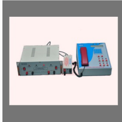
Level Crossing Gate Communication Equipment: TC 49
