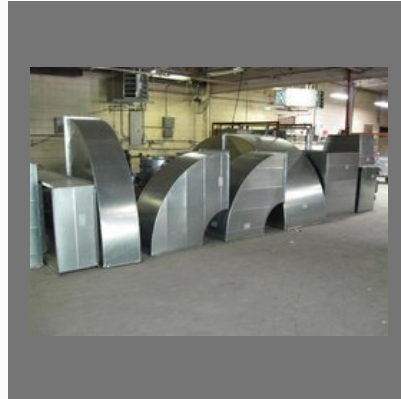
G I Duct
