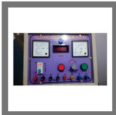
Thyristor Control Panel
