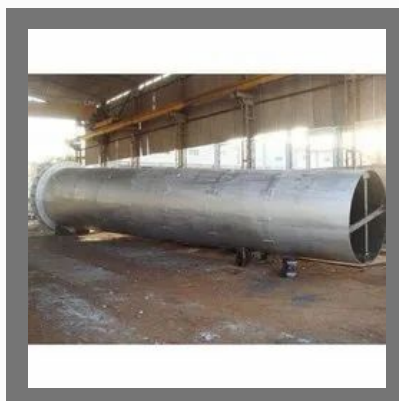
Self Supported Chimney
