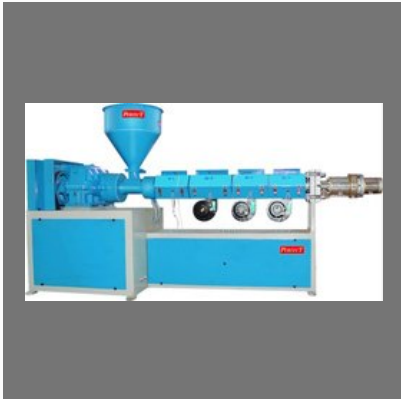
HDPE Pipe Machine
