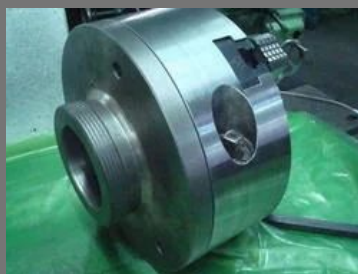
Worm & Worm Wheel Operated Self Centering Chuck
