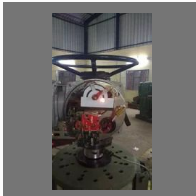
Torque Testing Of Pneumatic Actuator
