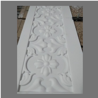
Solid Surface Router Cutting Work
