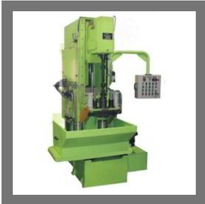
Honing Machine Reconditioning
