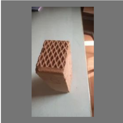
Wire cut bricks lines
