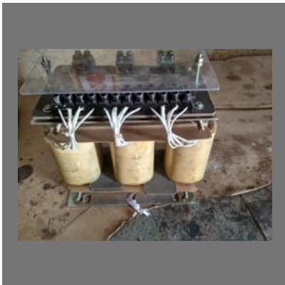
Three Phase Control Transformer
