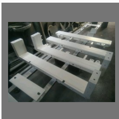
MS Transformer Structural works
