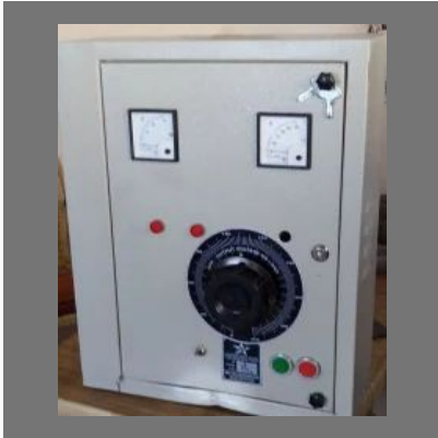
DC Control Panel
