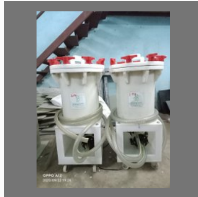
Electroplating Filter Unit
