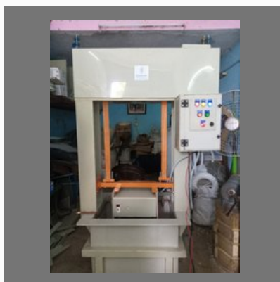
Semi Automatic Plating Barrel
