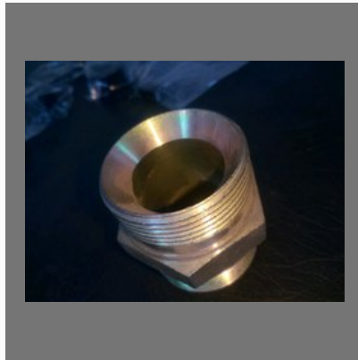
CNC Pipe Junction
