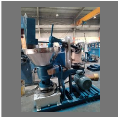
Rotary Chekku (Iron) Oil Extraction Machine 20 Kg With 10HP Motor (3 Phase)
