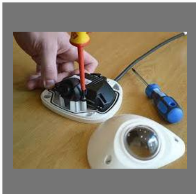
CCTV Camera AMC Service
