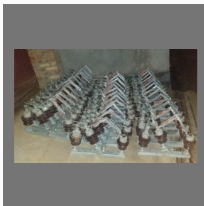
Air Break Switches
