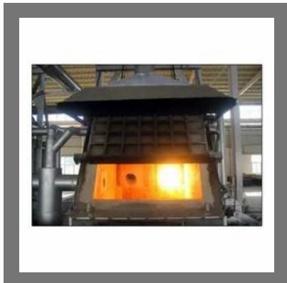
Aluminum Melting Furnace
