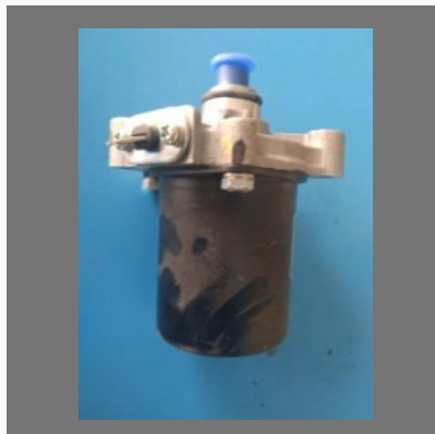
Self Pump Motor
