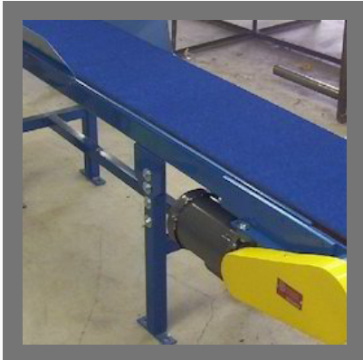
Belt Conveyor for Material Handling
