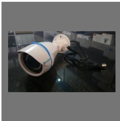
Bullet CCTV Camera
