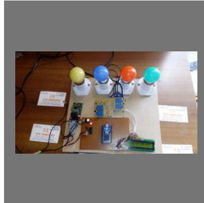
Wireless Bluetooth Based Smart Home Control System
