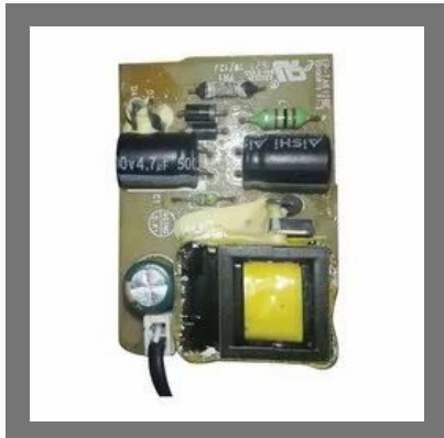
DC Power Supply
