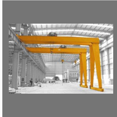
Semi Portal Crane
