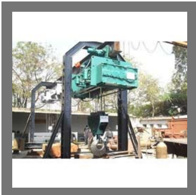
Electric Hoist Cranes
