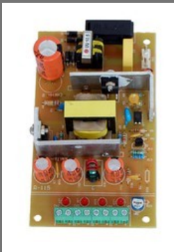
4 Channel CCTV Power Supplies
