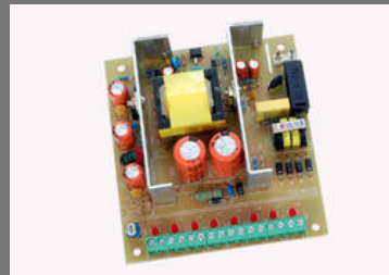
8 Channel CCTV Power Supply
