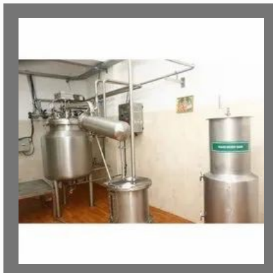
Herbal Distillation Plant
