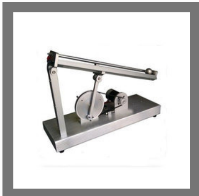
Ball & Beam Control System
