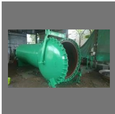
Autoclave for AAC Plant
