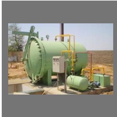
Timber Treatment Plant
