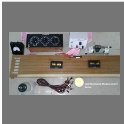
OSAW Leclanche Cell Resistance Measurement Setup
