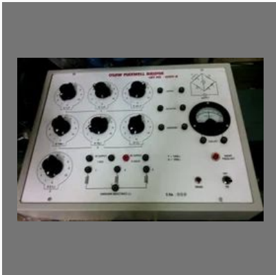
OSAW Maxwell's Bridge
