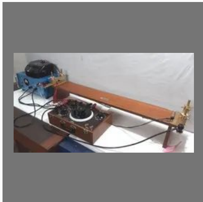
Osaw Senior Kelvin Double Bridge Setup
