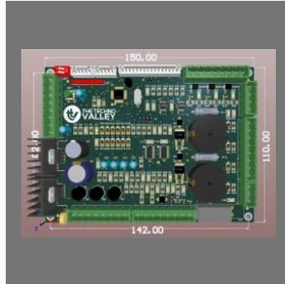
Magnetic Particle Inspection Control Board
