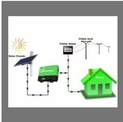
On Grid Solar System
