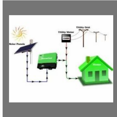
On Grid Solar System
