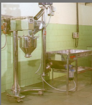
Broken Biscuit Handling System
