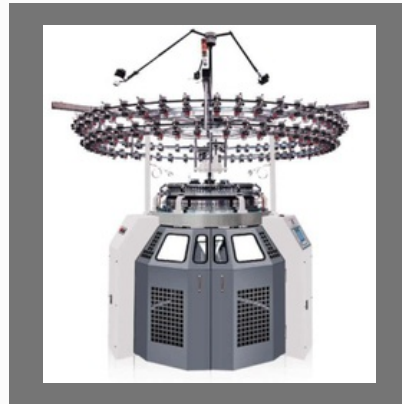
K-KNIT High Speed Circular Knitting Machine - Single Jersey 4 Tracks - Open Width : KK-SC
