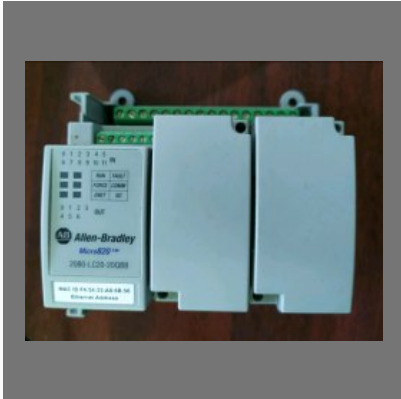
Allen Bradley PLC
