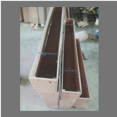
Submersible Pump Box
