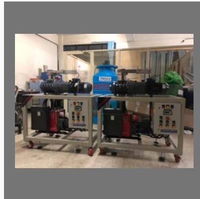
Rotary Roots Pumping System
