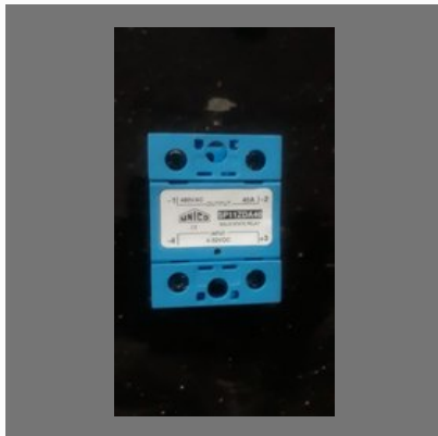
DC To AC Single Phase Solid State Relay SP11ZDA40
