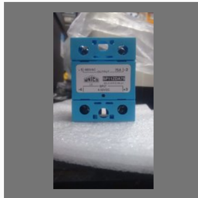
DC To AC Single Phase Solid State Relay SP11ZDA75
