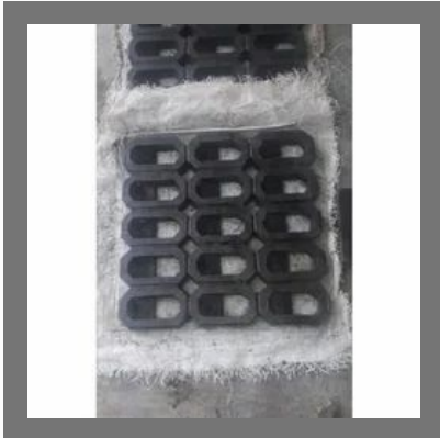
Decorative Concrete RCC Jaali
