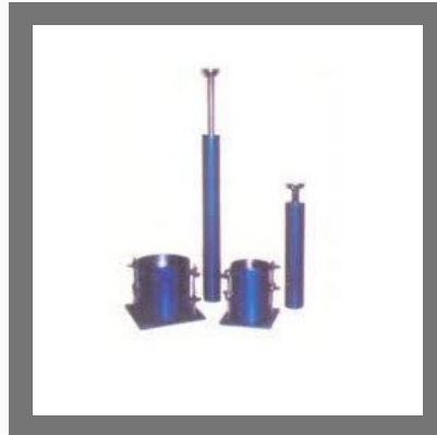
Compaction Test Apparatus
